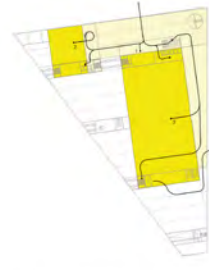
5. Access and flows - Conf. Halls (1) access from the street via main entrance, (2) access to the small conf. situated on Gt. +1, +2, (3) access to main conf. hall on 1st floor via the foyer, (4) outside extension on the galerie
